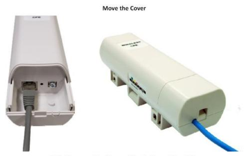
Slide the cover back to seal the bottom of the CPE.
