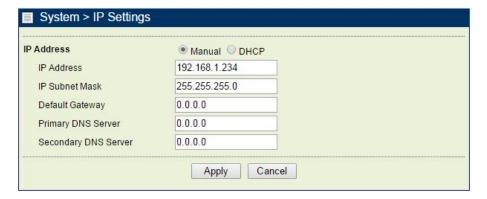
**IP Address:** Type the IP address you want to set to your Lite 5GHz MIMO HT-OFDM Outdoor radio (Default: 192.168.1.1).
