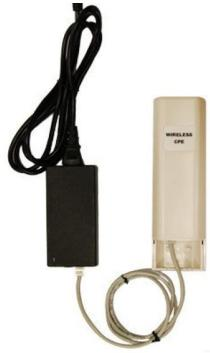
3. Connect the power plug to a power socket. The Lite 5GHz 2x2 MIMO HT-OFDM Radio will be powered up immediately.
