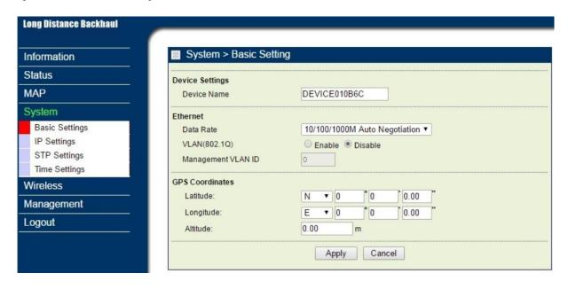
The **Device Name** is used to give a name to your 5GHz 4x4 MIMO HT-OFDM MESH Radio. This will enable you to manage your radio more easily if there are many radios in your network.
